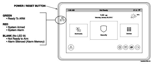
To reset the Touchscreen, press and hold the side Power Button for 3 seconds and then touch the "Press here to Reset" message on the screen to start the reset function. The Touchscreen can also be reset by pressing and holding the reset button for approximately 15 seconds until the touchscreen resets automatically.
